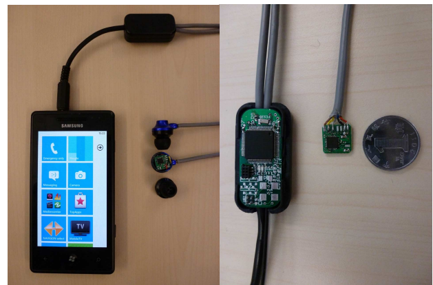
Figure 1. SEPTIMU hardware: the larger board is the baseboard ( 3.4 \times 1.4 \text{ cm}^2 ), and the smaller board is the sensor board embedded in earphones ( 1 \times 1 \text{ cm}^2 ).
