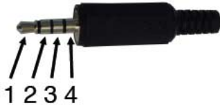
Figure 2. Audio plug and pin. The pin connections are: (1) left earphone (tip), (2) right earphone (ring), (3) common/ground (ring), and (4) microphone (sleeve).
